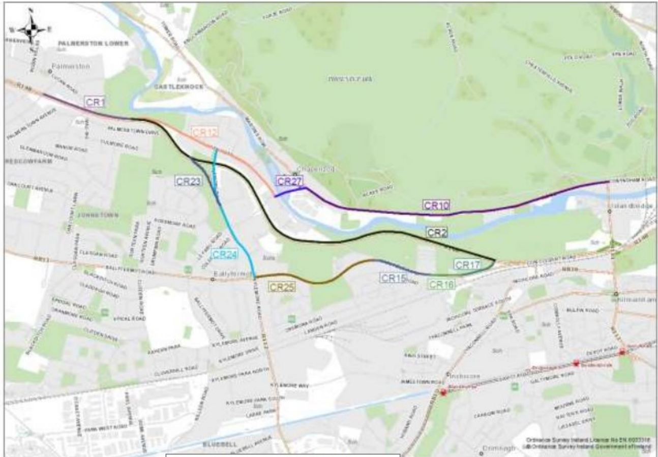
Image 3.11: Sub-Section SAS3 (Kennelsfort Road Upper to Con Colbert Road) Route Options extracted from the Feasibility Report
